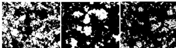
**Figure 5.** Phase masks for Mt Airy granite from hyperspectral analysis. (a) Plagioclase. (b) Quartz. (c) Orthoclase
