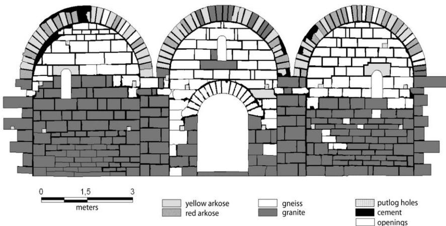
**Figure 4.** Lithological nature of stones based on stone-by-stone surveys.
