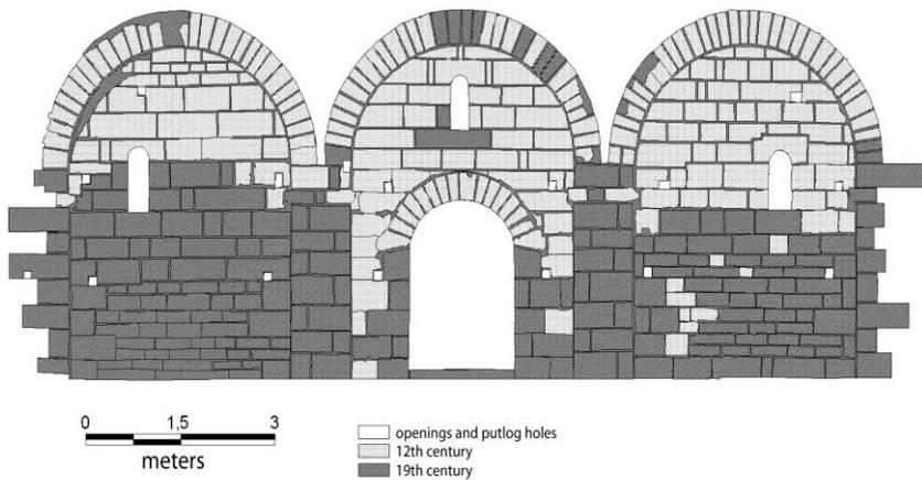
**Figure 3.** Differentiation between historic and replaced stones based on stone-by-stone surveys.
