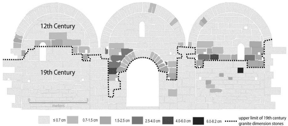
**Figure 5.** Accelerated stone recession just above the underpinned part of the arches based on 3D-modeling of stone decay by laser scanning.
