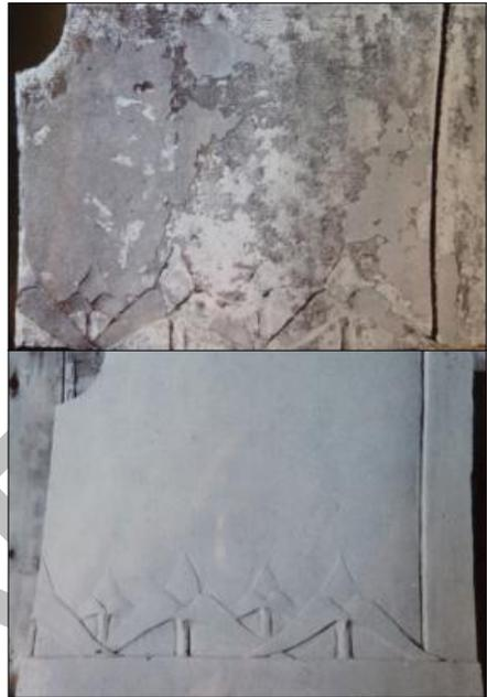
**Figure 4, 5.** Panel encrusted with calcium and magnesium deposits before treatment (above) and after successful ultrasonic cleaning (below).
