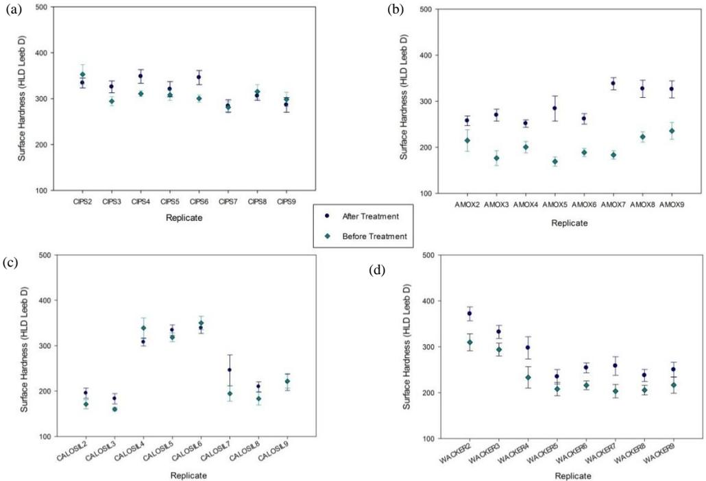
**Figure 1:** Graphs (a) – (d) to show change in surface hardness as measured by Equotip. (a) CIPS replicates; (b) AmOx replicates; (c) CaLoSil replicates; (d) Wacker replicates.
