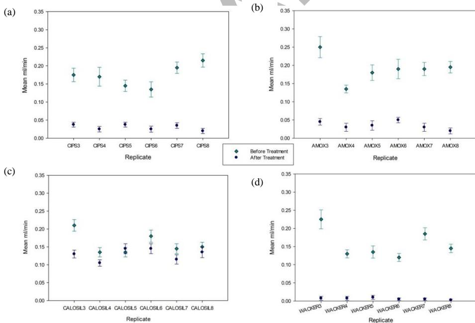
**Figure 2(a-d):** Graphs to show change in mean ml/min water penetration of replicates before (u) and after (l) treatment. (a) CIPS replicates; (b) AmOx replicates; (c) CaLoSil replicates; (d) Wacker replicates.
