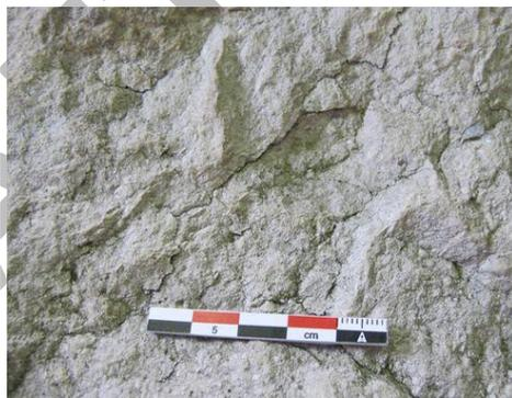
**Figure 5.** Back details of the limestone detached from the cornice
