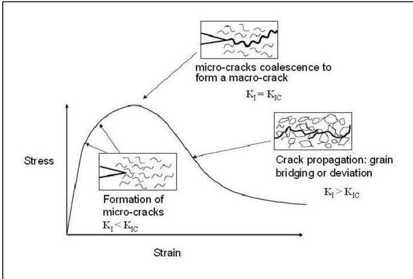
**Figure 2.** Cracks propagation into a porous substrate from micro-cracks formation to their coalescence into a main crack, and its propagation until failure of the specimen.
