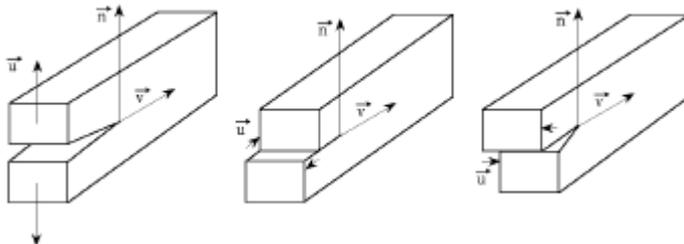
**Figure 3.** The three modes of crack-tip propagation. From left to right: mode I (tensile, opening); mode II (shear, in-plane sliding); mode III (tearing, out-of-plane sliding)
