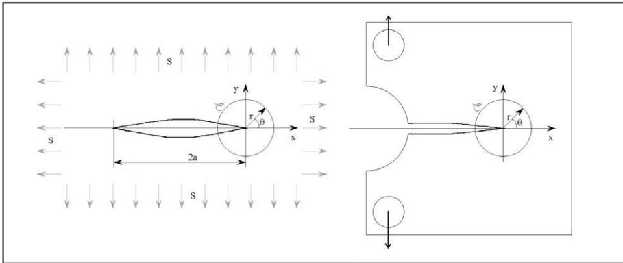
**Figure 1.** Cracks reference after Griffith and cordoned system at crack head (Griffith, 1921). On the right hand side, crack head is isolated in a sample test to be characterized.
