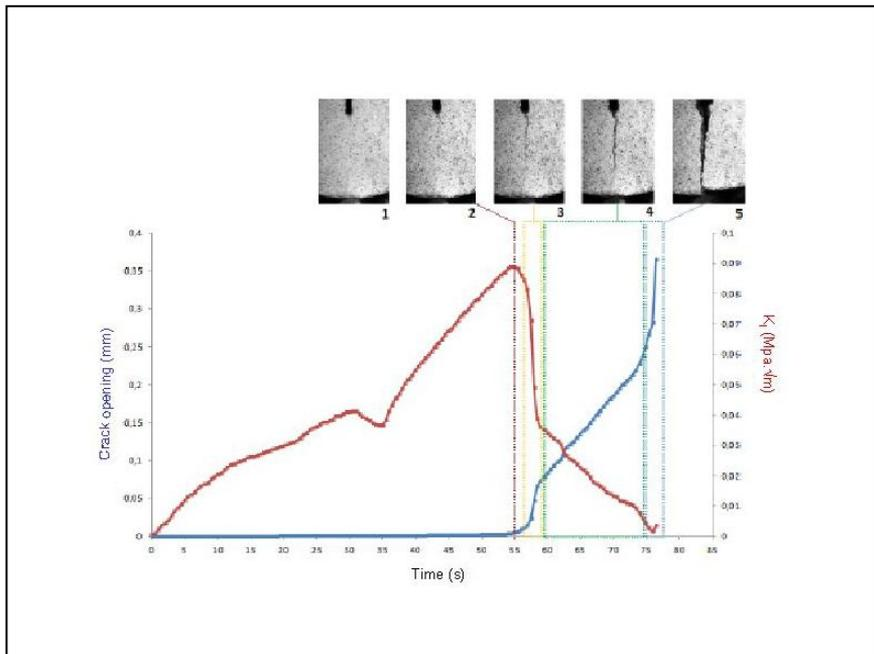
**Figure 7.** Evolution of crack opening and stress intensity factor as a function of time for a experiment of SCB type.
