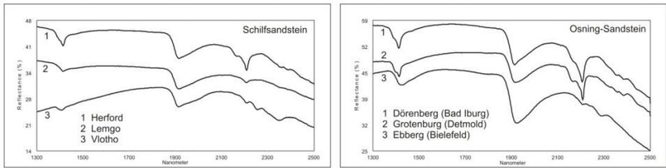
**Figure 4.** NIR-Spectra of Schilfsandstein and Osning-Sandstein from different regions in Westphalia (Germany) and
