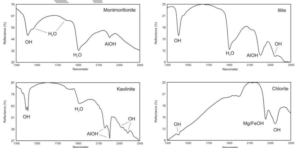
Figure 1. NIR-spectra of important clay minerals in sandstones
