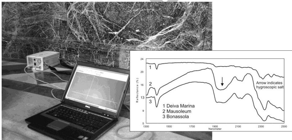
**Figure 7.** Investigation of serpentinite in the Kaiser-Wilhelm-Mausoleum in Potsdam. Good correlation with a sample of Bonassola. In comparison a sample from Deiva Marina
