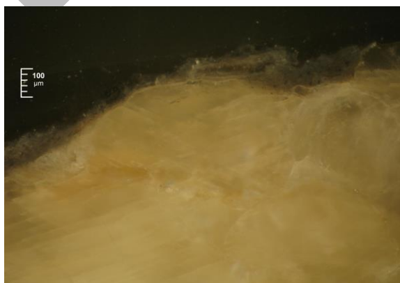
Fig. 3. Cross-section of a sample taken in the 1970s from the statue of St. Ambrogio (main portal).
