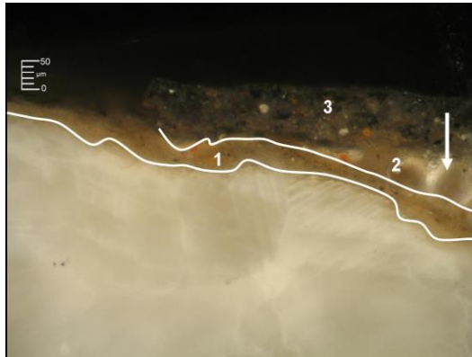
Fig. 4. Cross-section of a sample taken in 2010 from the statue of St. Ambrogio: 1- light brown patina (30 \mu\text{m} ), 2- non-colored layer with gypsum, siloxane and acrylic resin (some glass spheres are visible on the right), 3- top black layer.
