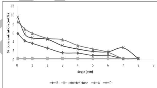
**Figure 8.** Distribution profile of Si within the stone by EDS analyses with reference to the each treatment.
