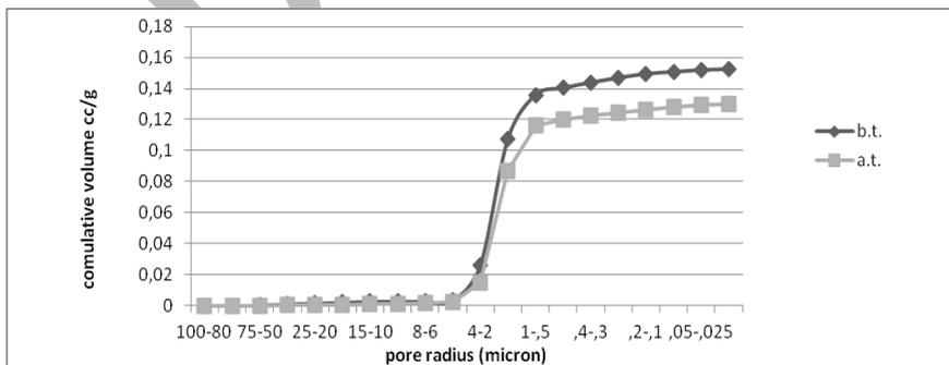
Figure 10. Cumulative volume curve at the depth's interval 0-0.5 cm
