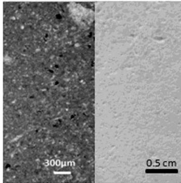
**Figure 1.** GS medium-fine calcarenite [wackestone, thin section photomicrograph, polarised light, crossed nicols (left); macrophotograph (right)]
