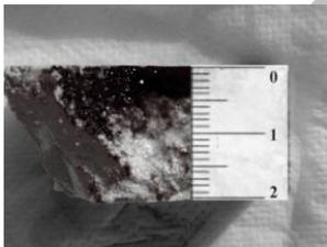
**Figure 7.** Depth of penetration by the phenolphthalein color test (Treatment A)
