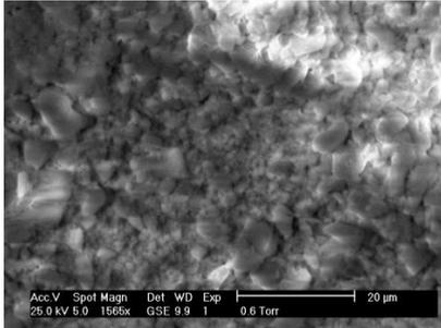
**Figure 2.** Untreated stone surface
