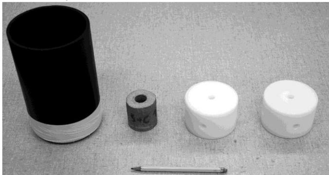
**Figure 1.** The parts of the setup used for maintaining wet and under the load applied by the testing machine the core-drilled stone samples. From right to left, two drilled discs in polyoxomethylene to be placed on the top and on the bottom of the sample. The holes allow the water to get easily
