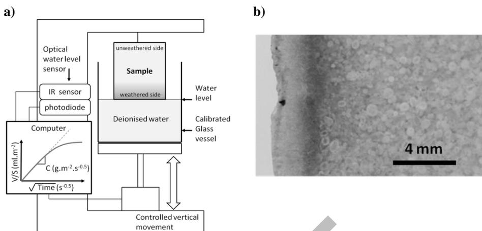
**Figure 1.** a) Scheme of the used automatic monitoring soaked volume for capillarity measurement. Here the sample is positioned for the weathered side capillarity measurement. b) Microphotograph showing a colonised patina on sample MC1 (Roman temple Maison Carrée).
