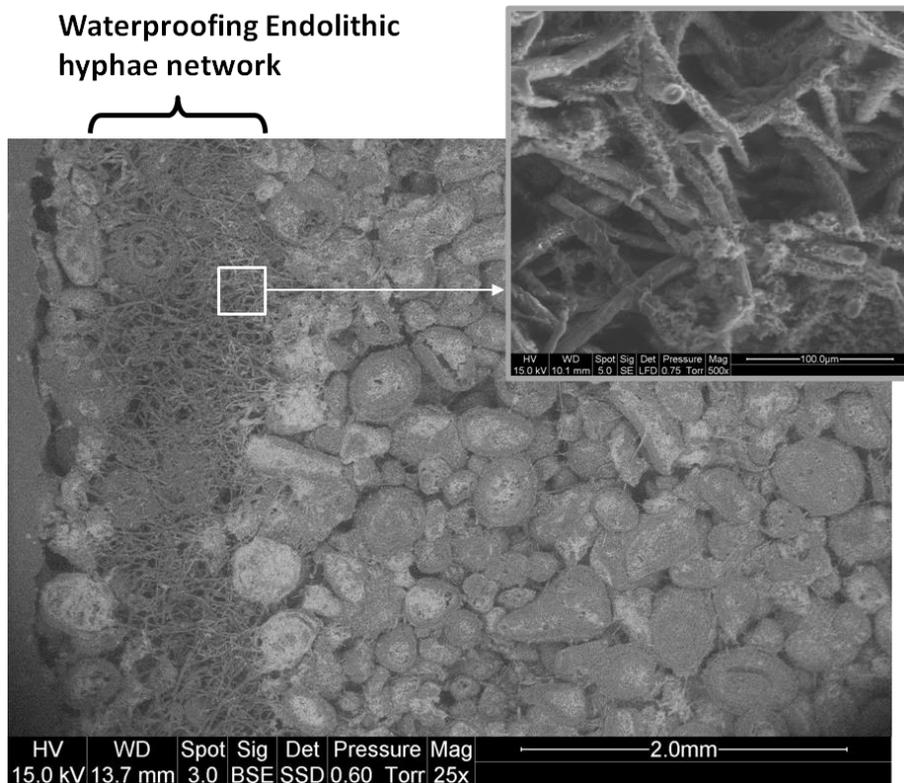
**Figure 2.** SEM of the moulded porous network showing a secondary porosity due to growth of endolithic lichen hyphae on sample MC1 (Roman temple Maison Carrée).
