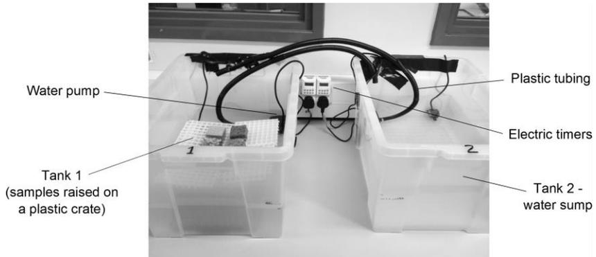
**Figure 1.** Experimental set-up used to simulate intertidal conditions in the laboratory.
