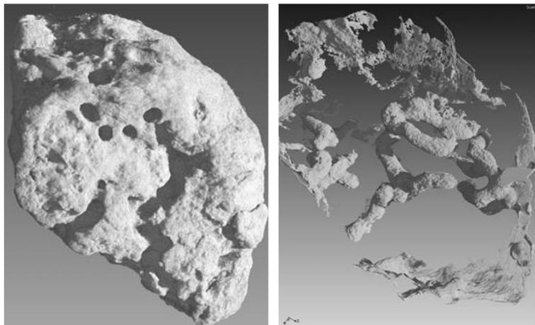
**Figure 9.** Ferruginous sandstone block (size: 12x6x8 cm), CT-scan of the block (left) and negative-density 3D-reconstruction showing the internal distribution and connectivity of the burrows dug by mason bees (right).
