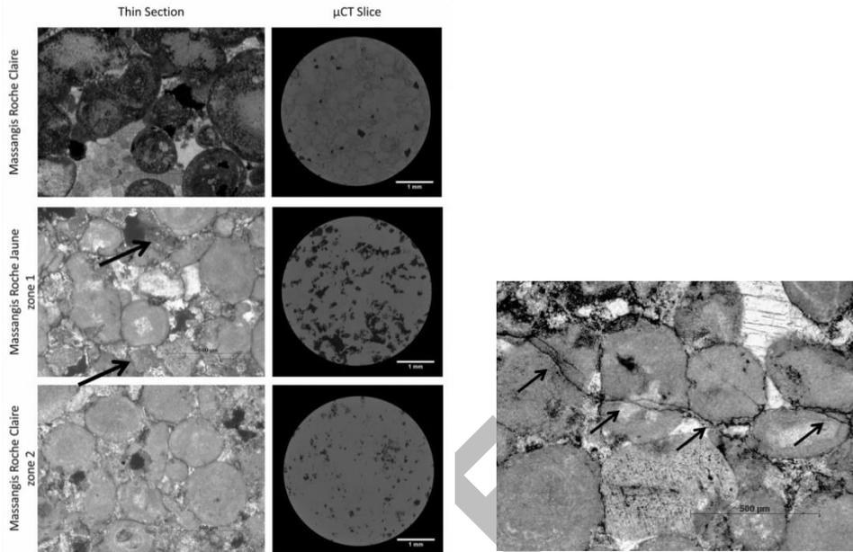
**Figure 1.** Left: thin sections and  $\mu$ CT slices of Massangis Roche Claire, Roche Jaune zone 1 and 2. Right: Cemented fissure crosscutting Massangis Roche Jaune
