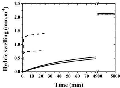
**Fig. 4** Hydric swelling of the natural stone (dash line) and the artificial stone (full line).
