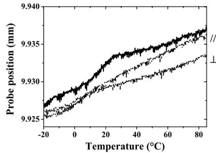
**Fig. 5** Thermal expansion of the artificial stone (full line) and the natural stone (dash line). The dependency of the thermal expansion with the bedding for the natural stone is reported.
