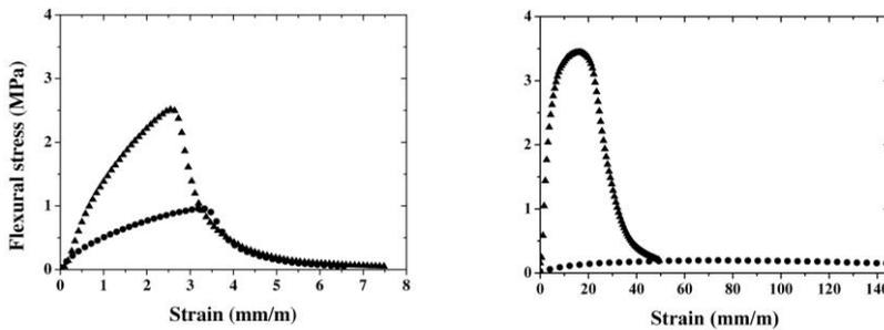
**Fig. 6** Strain-stress curves of the natural stone (left) and the artificial stone (right). The triangles represent the dry state while the circles represent the wet state.
