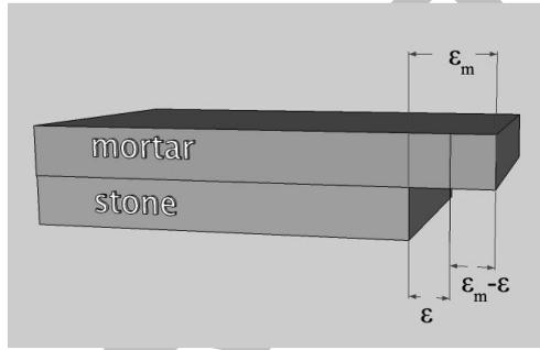
**Fig. 7** The expansion of the mortar and the induced expansion  $\varepsilon$  of the underlying stone.
