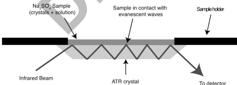
**Figure 2:** Protocol device used for FTIR-ATR spectroscopy. Droplet of  $\text{Na}_2\text{SO}_4$  solution is put directly on the ATR crystal.
