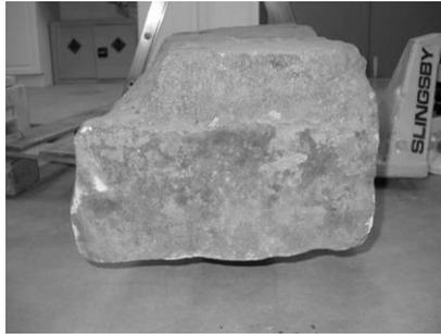
**Figure 2.** Uneven bottom surface of memorial stone
