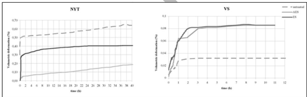
**Figure 2** Volumetric dilatation of NYT and VS, both untreated and treated.
