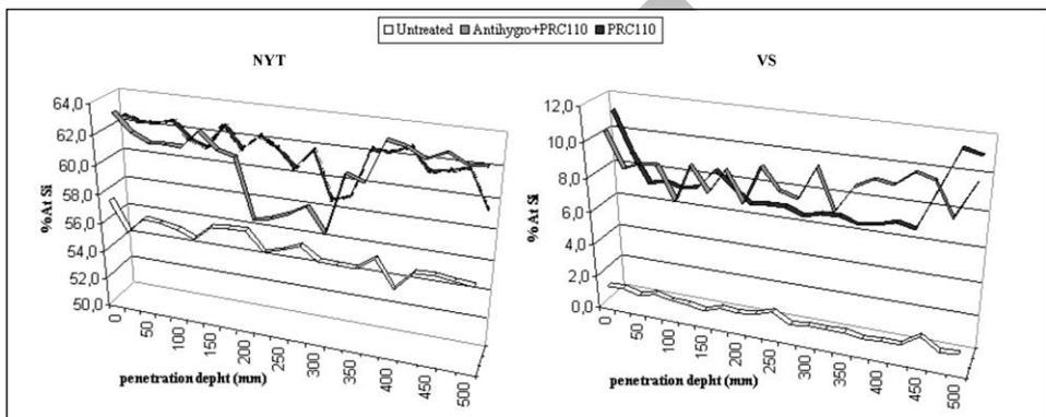
**Figure 1** Profiles of the Si concentration (in atomic percent) along the cross section of NYT (left) and VS (right) specimens both untreated and treated.
