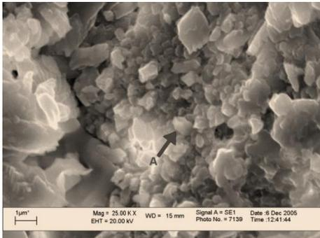
**Figure 2.** Naturally weathered non-desalinated sample untreated (left)
