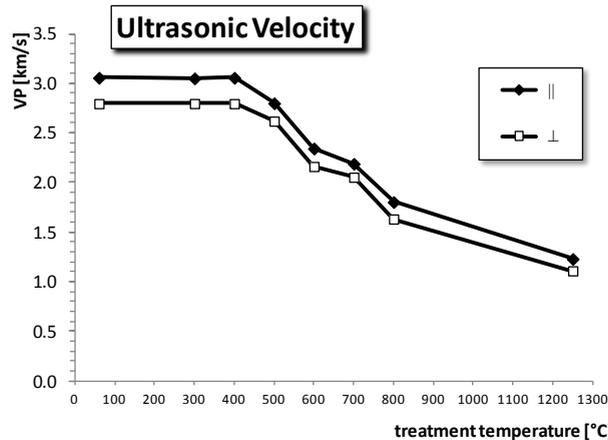
**Figure 12.** Ultrasonic Velocity decreases significantly ( $\perp$  = normal to bedding,  $\parallel$  = parallel to bedding).
