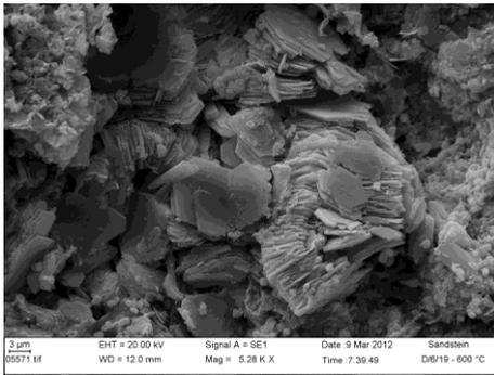
**Figure 6.** Treated at 600°C, undisturbed booklets of kaolinite
