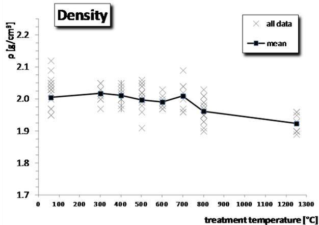
Figure 10. Density development of the sandstone, all measured data and calculated mean.
