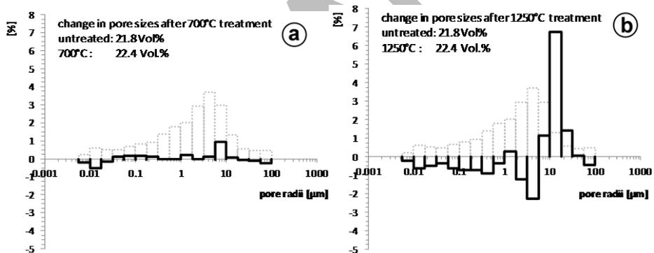
**Figure 9.** Change in pore size distribution according to temperature treatment. Dotted lines show untreated material, black lines show the difference of the treated material relative to the untreated. a) 700°C, b) 1250°C. Portion of smaller pores is reduced in support of larger pores.
