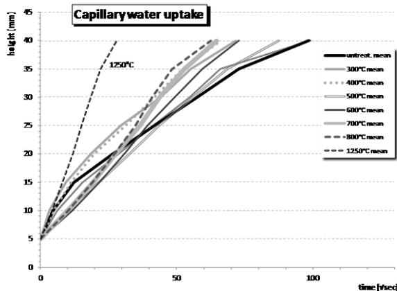
**Figure 8.** Capillary water uptake is accelerated
