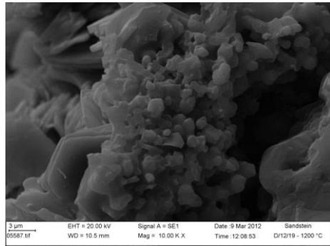
**Figure 7.** Melting structures and pseudomorphs of kaolinite at 1250°C
