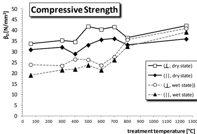
Figure 11. Compressive strength data, parallel and normal to the sedimentary bedding.
