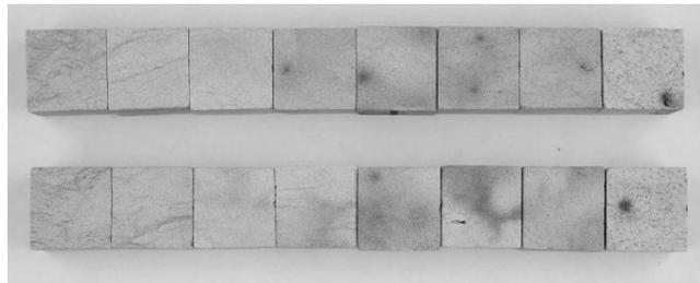
**Figure 5.** Samples from left to right: untreated sample (grey), 300°C (yellow touch); 400°C (yellow clouds); 500°C (pale red); 600°C (red); 700°C (dark red); 800°C (dark red); 1250°C (grey)
