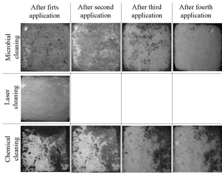
**Figure 4.** Sequence images of cleaning applications on the Carrara marble column.
