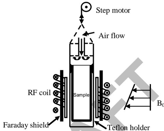
**Figure 4.** A schematic diagram of the NMR set-up used for spray drying experiments
