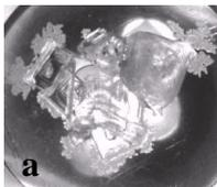
**Figure 3.** Images showing the crystal morphology at the end of droplet drying experiment (a) with no inhibitor (b) 0.001 m inhibitor (c) 0.01 m inhibitor. These images are captured using dino-lite digital microscope.
