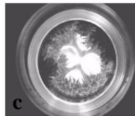
showing the crystal morphology at the end of droplet drying experiment (a) with no inhibitor (b) 0.001 m inhibitor (c) 0.01 m inhibitor. These images are captured using dino-lite digital microscope.
