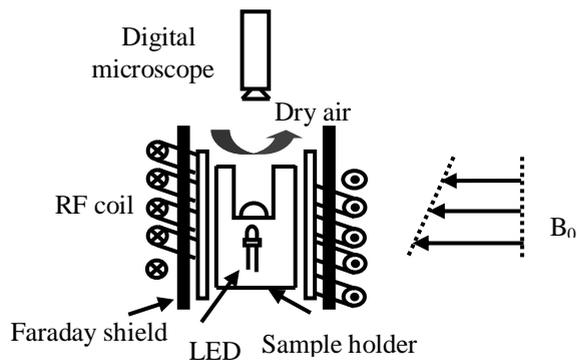
**Figure 1.** A schematic diagram of the NMR set-up used for droplet drying experiments
