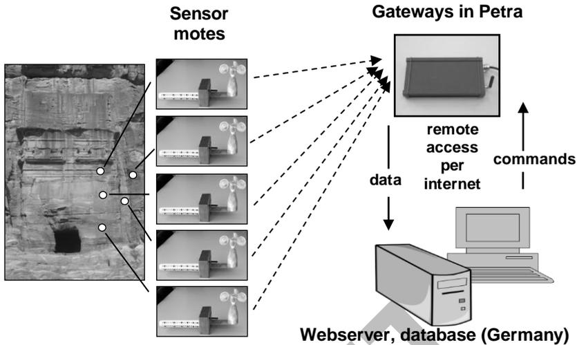
**Figure 12.** Configuration of the wireless sensor network, data transfer from the sensor motes via gateways per internet to remote webservice / database
