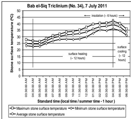
**Figure 9.** Bab el-Siq Triclinium, stone surface temperatures in high summer (example), façade exposed to NW
