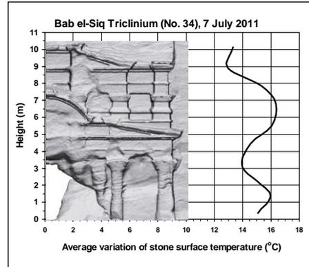
**Figure 10.** Bab el-Siq Triclinium, average diurnal variation of stone surface temperatures (vertical profile) in high summer (example)
