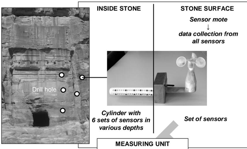
**Figure 11.** Configuration of the wireless sensor network, measuring unit with sets of sensors and sensor mote for data collection
