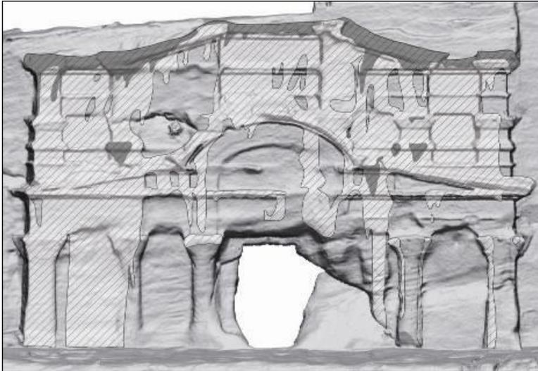
**Figure 8.** Bab el-Siq Triclinium, 3D image with documentation of water run-off, dark gray areas with hatching: water run-off after light / short rain, light gray areas with hatching: additional areas by water run-off after heavy / long rain
