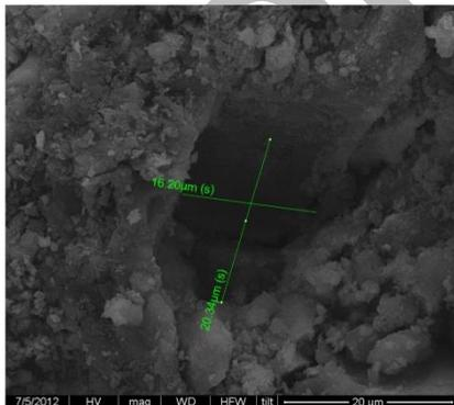
**Figure 5.** SEM image of treated with PMC stone from Rhodes. Image indicates the pore diameter, Bar = 20 μm
