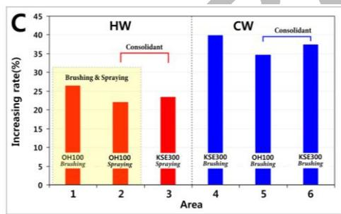
Figure 3. (C) Increased ultrasonic velocity by consolidants and application methods
