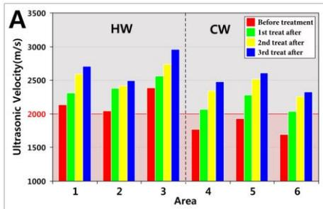
Figure 3. (A) Ultrasonic velocity during and after in-situ consolidation of sandstone. Ultrasonic velocity by application areas during the consolidation
