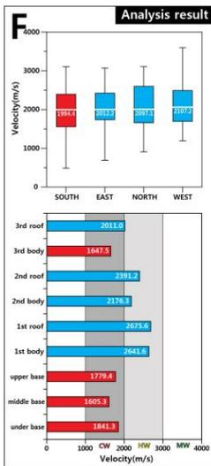
Figure 1. (F) Average ultrasonic velocity according to the elevated position of the stone elements
