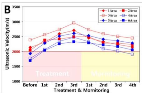
Figure 3. (B) Ultrasonic velocity by application areas during the consolidation
