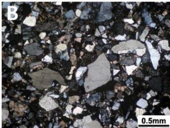
**Figure 1. (B)** Polarizing microscopic images showing heterogeneous roundness and grading of quartz
