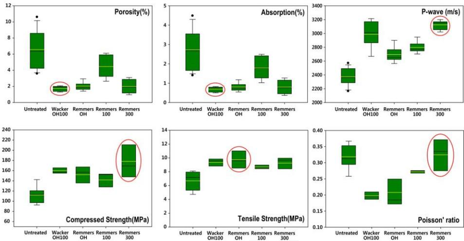
**Figure 2.** Physical properties of the untreated and treated samples by consolidants
