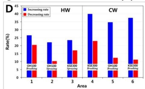
**Figure 3. (D)** Ultrasonic velocity change during and after the consolidation
