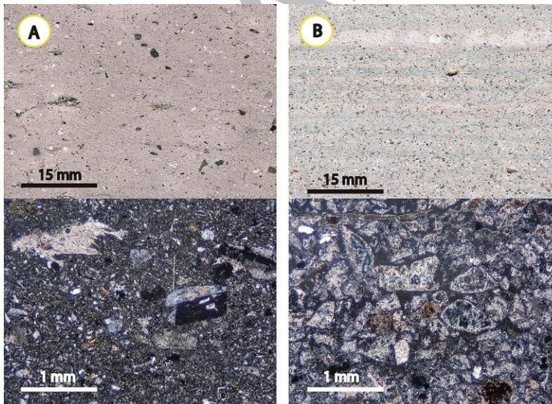
**Figure 2.** Thin section photomicrographs of the studied rocks. A: Trachytic porphyritic texture of the Bufa rhyolite, where are embedded subhedral to euhedral quartz and plagioclase crystals in a microcrystalline and partially devitrified glassy matrix. B: The Loseros tuff shows a matrix that is made up of opaque components (volcanic glass) with small crystals of calcite and altered plagioclase (albite).
