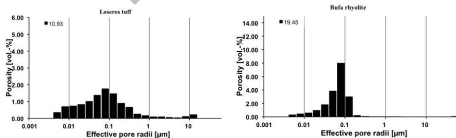
**Figure 3.** Histograms showing the relationship between the porosity and the pore radius of the Loseros tuff (left) and Bufa rhyolite (right).
