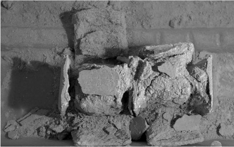
**Figure 2.** The destruction of the samples of the Roman cement repair mortar with setting retarder, the second cycle of the resistance to the soluble salts examination
