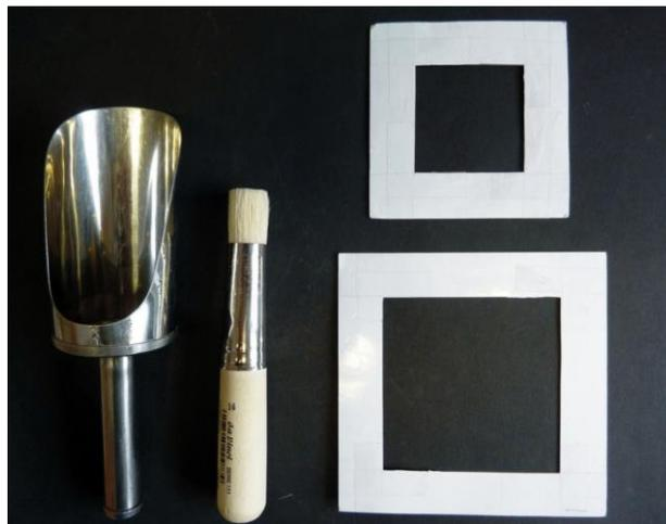
Figure 2. Utensils for the abrasion test
