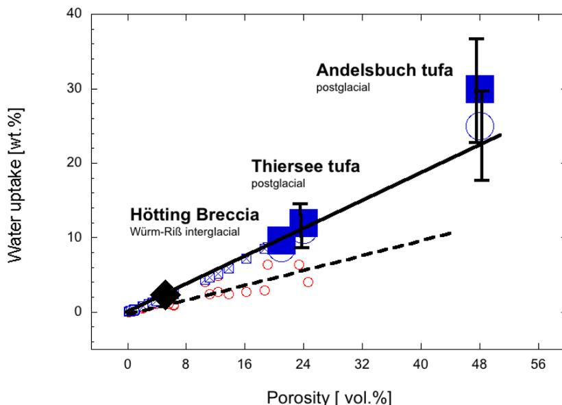
**Figure 4.** Plot of the water uptake (wt%) and pore volume (vol.%) of different limestones (Grimm, 1990) (small circles and squares), Gröden sandstone (closed diamond) and the studied quaternary sediments of Hötting breccia, Thiersee and Andelsbuch tufa (closed squares). While the open symbols represent water uptake at atmosphere condition, closed symbols give the uptake under vacuum. (Note: the data of the quaternary materials have been converted from vol.% to wt.%; cf. Table 1).
