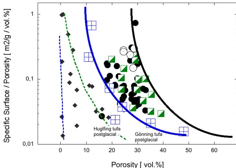
**Figure 6.** Plot of (specific surface/porosity) vs. porosity (cf. Fig. 5) with compilation of additional data of medieval lime mortars from three localities. The data of these “youngest sediments” plot on the high porosity side of the diagram indicating a similar trend as observed for the quaternary
