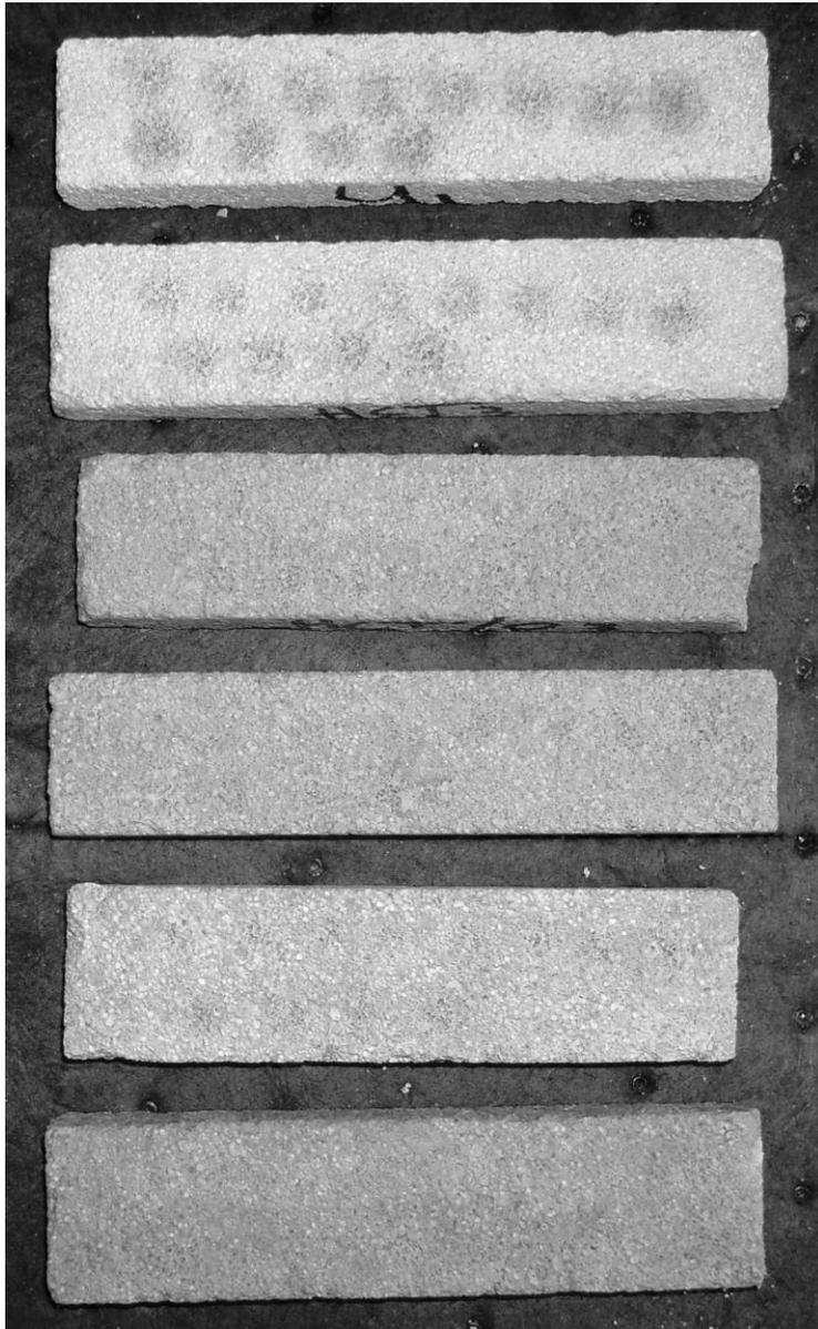
**Figure 1.** Limestone after Phillips Microabrasion Testing. From top to bottom: Untreated Control, HCT, HCT/OH100, OH100, T-2333, and T-2333/OH100.
