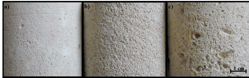
Figure 1. Fine-grained (a), medium-grained (b) and coarse-grained (c) limestone
