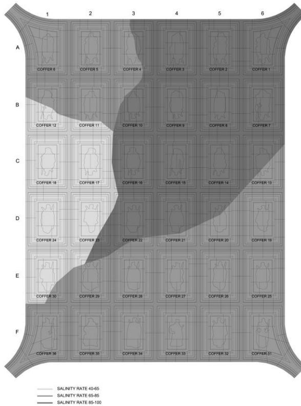
Figure 5. Salinity in the stone of the vault
