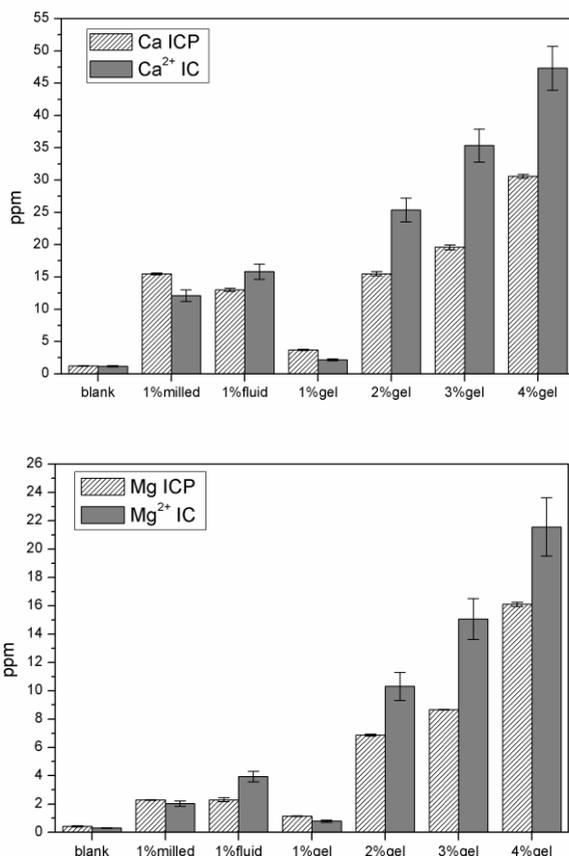
**Fig. 7.** Comparison between results of calcium and magnesium detected by means of IC and ICP-AES.
