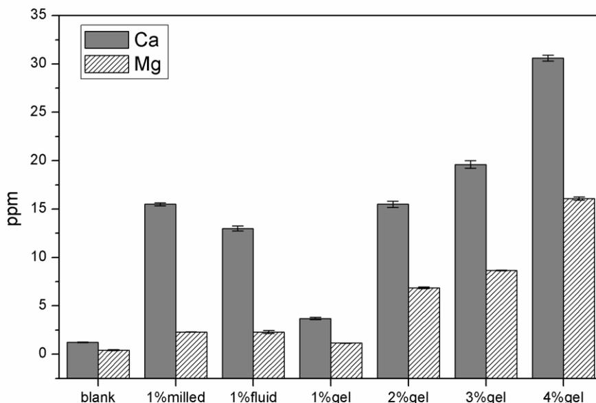
**Fig. 6.** Concentrations ( $\mu\text{g}/\text{ml}$ ) of  $\text{Mg}^{++}$  and  $\text{Ca}^{++}$  in aqueous solutions extracted from stone materials and recovered from agar samples prepared with different concentrations of agar (1-4 %) and in different modes (gelified, milled and fluid). Blank sample was used as comparison (see text).
