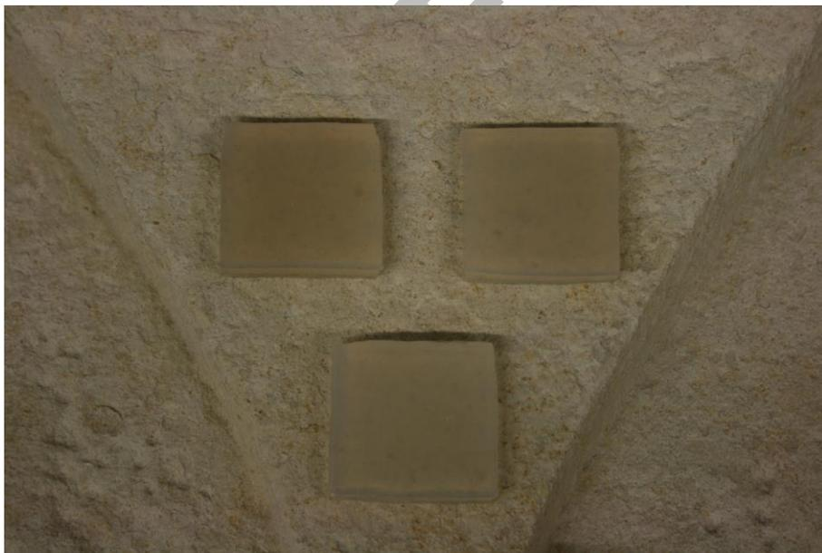
Fig. 3. Capital of Angera Dolostone during cleaning tests with agar gels 1,2,3 % concentration in water.
