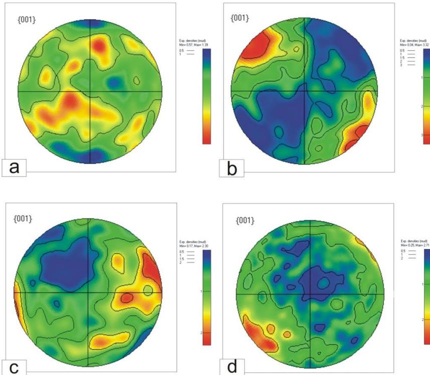
**Figure 3.** {001} Pole figures from the EBSD HKL Channel 5 software for marble samples in xz planes: **a.** Arabescato Altissimo (Carrara marble from Italy); **b.** Sölk (calcitic marble from Austria); **c.** Lasa (calcitic marble from Italy); **d.** HT-Carrara (Carrara marble from Italy).
