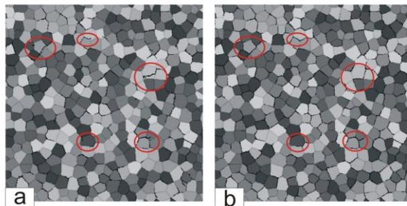
**Figure 7.** Simulations of microcracking in a dolomite marble with a grain size of 1 mm upon heating by a temperature differential of  $50 \text{ }^\circ\text{C}$ : **a.** equiaxed microstructure with random texture and
