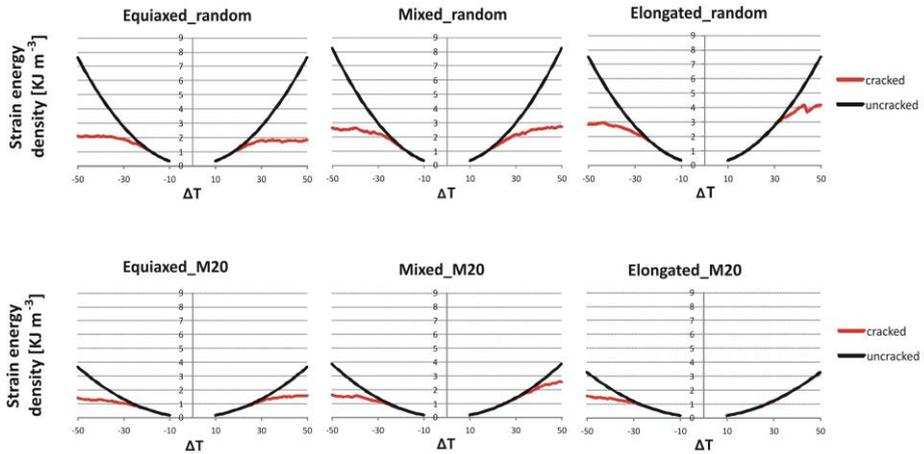
**Figure 4.** Elastic strain energy density for microcracked and uncracked idealized marble microstructures versus the temperature change from the unstressed state. Results are shown for three idealized calcitic microstructures (equiaxed grains; mixture of equiaxed and elongated grains; and elongated grains) and for two LPOs: random texture and 20 times random texture (denoted as M20) with a grain size of 1 mm and a grain boundary toughness  $0.40 \gamma_{\text{xtal}}$ .
