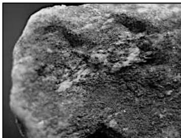
**Figure 12.** Photomicrograph of the deposition (case 1) on the surface of the marble
