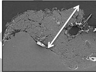
**Figure 11.** SEM photomicrograph of the encrustation. Small Al-Si grains can be identified. Clear limits with the substrate.
