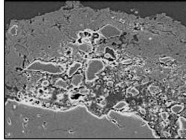
**Figure 5.** SEM photomicrograph of the deposition with the confined grains in the lower layer.
