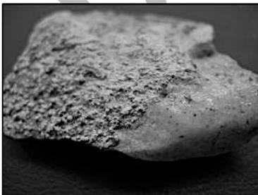
**Figure 6.** Photomacrograph of the encrustation (case 1) on the surface of the marble.
