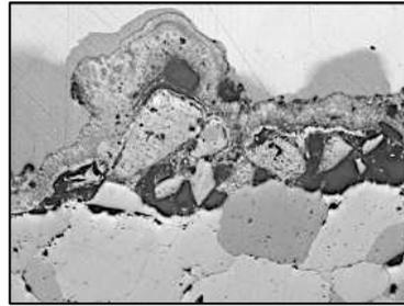
**Figure 9.** Light Microscopy //Nichols. Two deposition layers can be identified as well as the grains of calcite and quartz.
