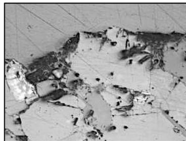
**Figure 13.** Light Microscopy //Nichols. Impregnations (black stains) of ferric and aluminosilicious
