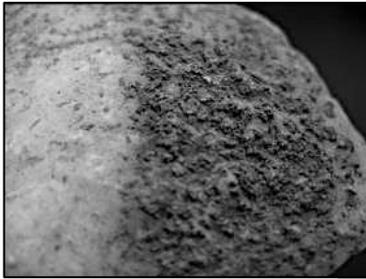
**Figure 10.** Photomicrograph of the encrustation (case 2) on the surface of the marble
