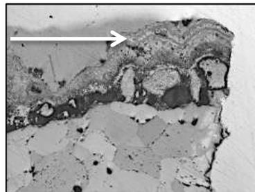
**Figure 7.** Light Microscopy //Nichols. Alternating deposition layers of calcite and quartz.
