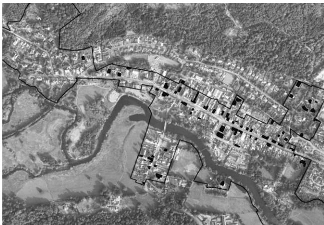
**Figure 6** GIS aerial base map of Callander Conservation Area displaying a cross query of all surveyed built sites with CONGLOMERATE walling and CEMENT POINTING AND PATCHING.
