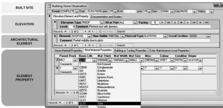
**Figure 2** Module input form, as seen on tablet PCs used during survey, with hierarchy labelled on left hand side. The form is used to enter data into the relational database. The number of elevations and elements are selected, and properties are recorded for each element using a number of pre-defined fields with supporting drop-down dictionaries.
