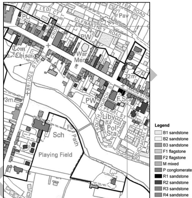
**Figure 5** GIS topographic base map of Callander town centre with coloured (in grey-scale) polygons representing surveyed sites displaying the distribution of stone types used in WALLING (left) and the distribution of slate types (right) used in ROOFING in the Callander Conservation Area. This map is typically viewed in colour (not grey-scale) to better differentiate the distribution of stone and slate types to the user.
