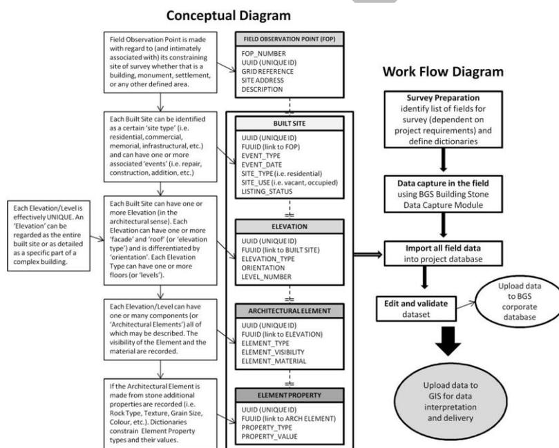
**Figure 4** The conceptual diagram defines the relationship of the data elements in the Building Stone Data Capture module and the structure between them. The Work Flow diagram defines the process of population and data delivery.
