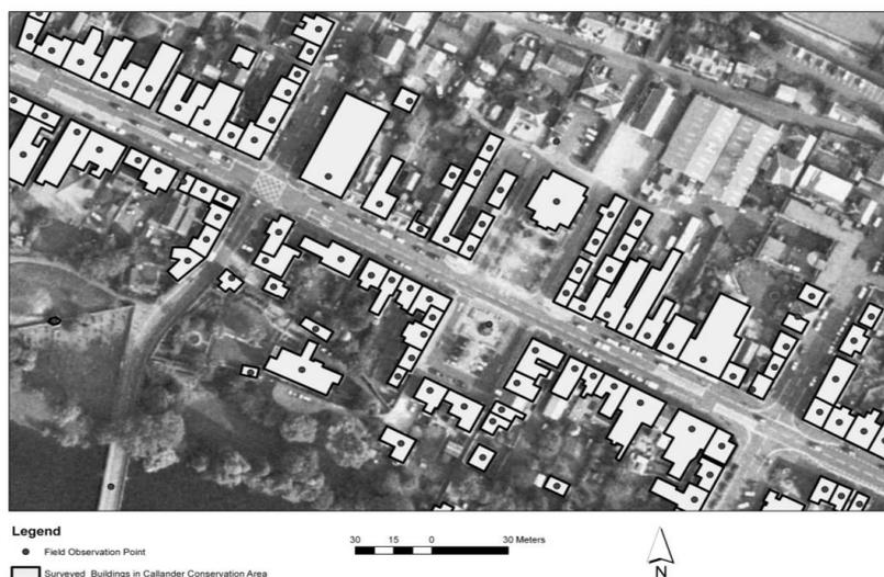
**Figure 3** GIS aerial base map with geo-referenced polygons representing the limits of each unique built site. Each polygon has a Field Observation Point, or unique reference number, used for identification and data attribution.
