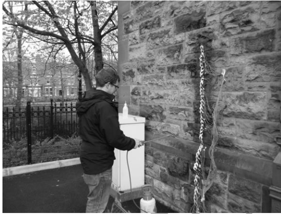
Figure 3. Monitoring moisture uptake on sandstone wall patchily covered with green algae using 2D resistivity surveys, Belfast, Northern Ireland.
