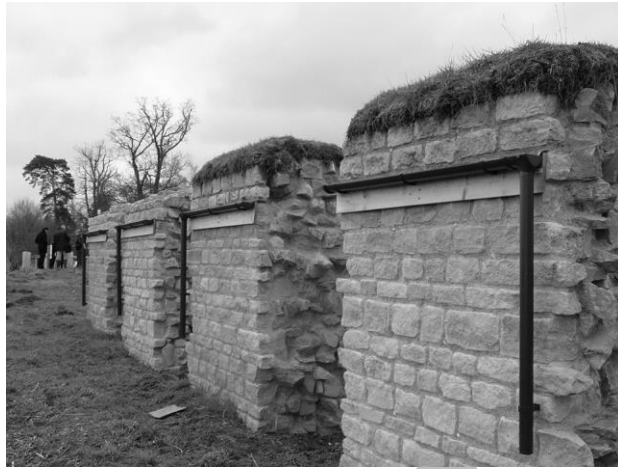
Figure 2. Soft and hard capped test walls, with gutters and down pipes to collect runoff, Wytham Woods, near Oxford, UK.
