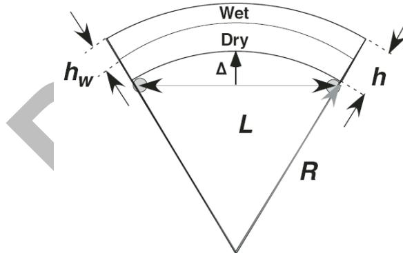
**Figure 1.** Geometry of warping experiment. Wet stone attempting to expand is compressed by dry stone, inducing deflection.
