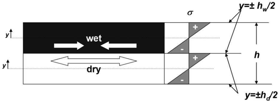
**Figure 6.** Schematic of stress in a plate of stone during the warping experiment, assuming linear elasticity.
