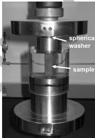
**Figure 3.** Experimental setup for swelling pressure experiments.
