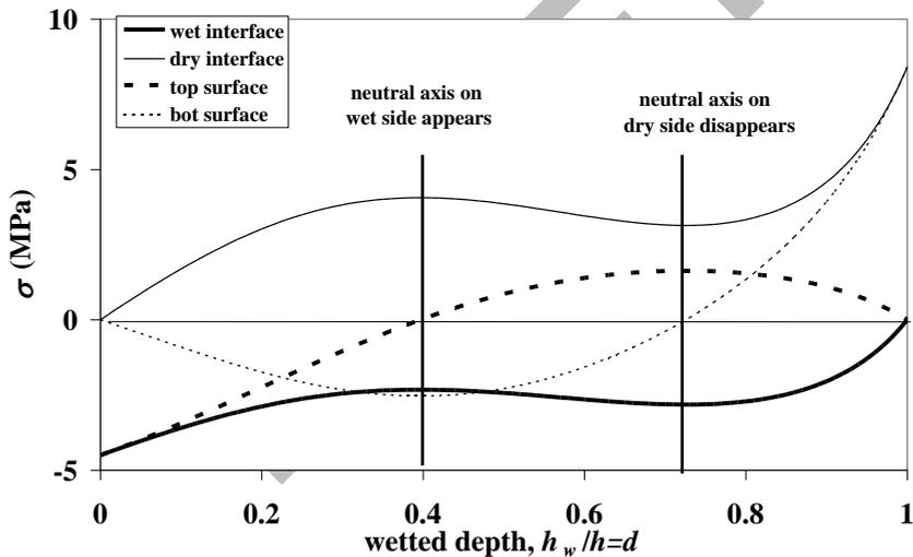
**Figure 7.** Stress in the wet and dry portions of the stone plate during a warping experiment as a function of wetted depth. The majority of the stress in the wet part of the stone is compressive for the duration of the experiment.
