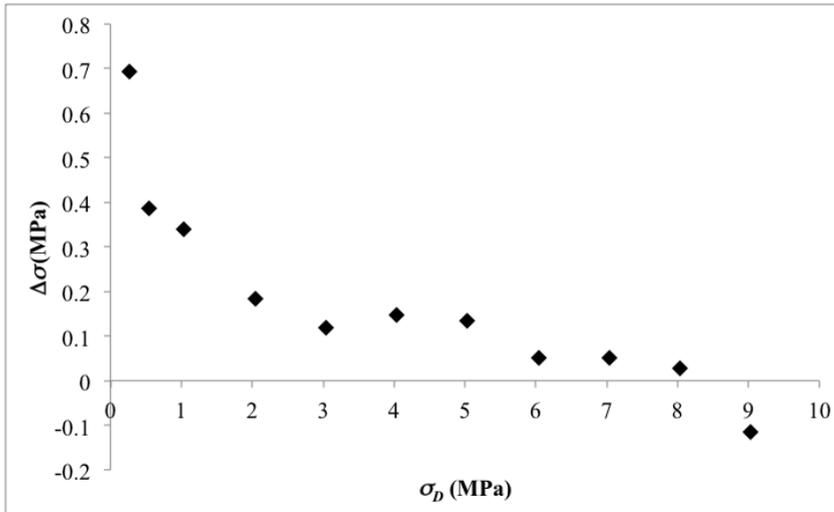
Figure 5. Change in pressure of stone upon saturation versus initial overburden stress  $\sigma_D$ .
