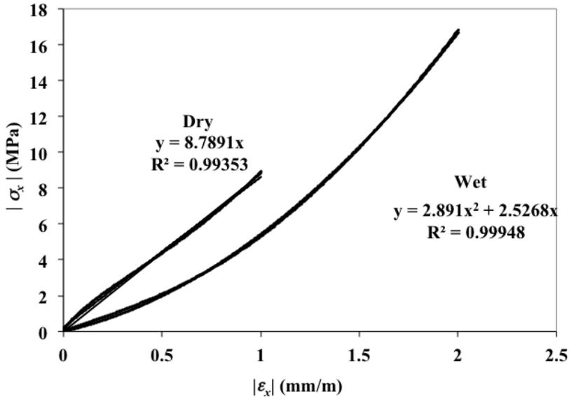
Figure 4. Stress-strain curves for Portland brownstone under compression in the wet and dry state.
