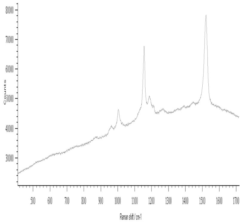
**Figure 2.** Raman spectrum showing characteristic peaks of the biomarker carotene, which provides protection for algal cells during photosynthesis.
