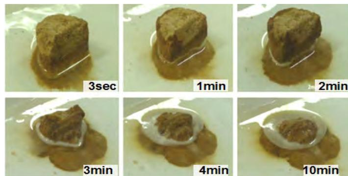
Figure 4 Collapse of stiff sand in water less than 10 min.
