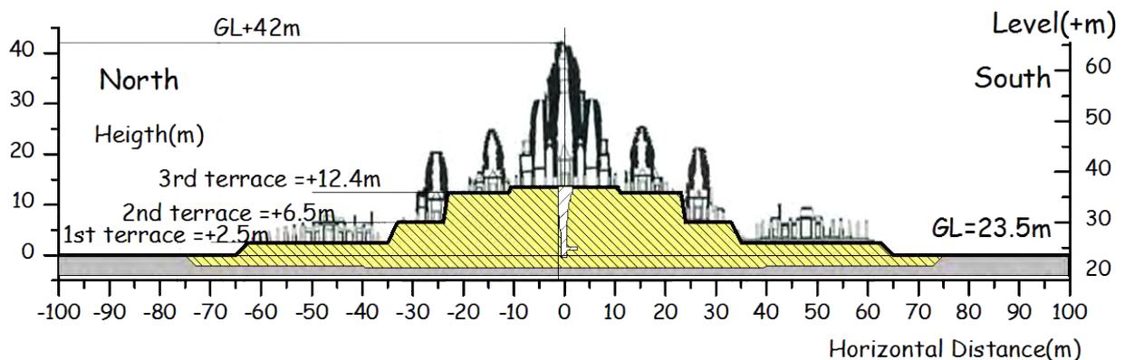
Figure\_2 Vertical Section of the sand filled mound, Bayon Temple
