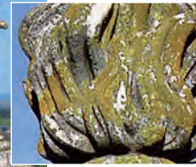
Folious lichen (Ramalina sp.) growing on a granite dimension stone.
